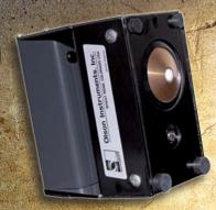
The CTG-2 is a hand-held, battery powered, nondestructive system for measuring the thickness and integrity of concrete slabs, pavements, tunnel linings, walls and other plate-like structures using the Impact Echo principle.
