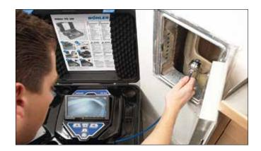
**Commercial & Residential Building Inspection** Detection of problems in hollow spaces, intermediate ceilings, ductwork and chimneys
