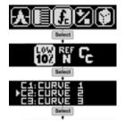
Reduced dispersion and direct conversion to compressive strength based on validated curves, regional curves or user defined curves bring improved accuracy to compressive strength estimates.
