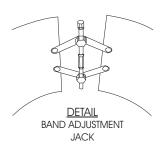
Use optional VSJ stainless steel Pipe Mounting Bands for easy Sensor installation in round pipes.
