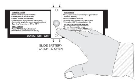
Use new, premium quality Alkaline D-Cell batteries only (Energizer E95 or Duracell/Procell MN1300).
