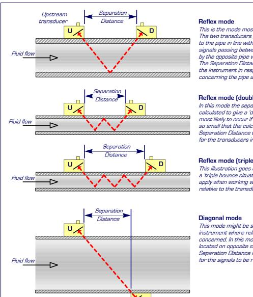
This is the mode most commonly used. The two transducers (U & D) are attached to the pipe in line with each other and the signals passing between them are reflected by the opposite pipe wall.
