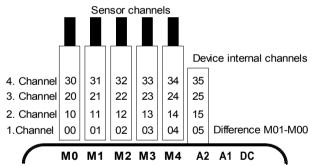
Once the range has been programmed the standard reference channels can be used (see above). Settings for the reference channels are described in 10.4.6. The best approach is to use the **Function channel** assistant.
