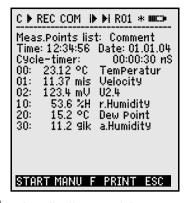
start the first measurement with the key <START> and cyclically record the measured values. If a printer or terminal is connected, all values are also put out online. After selecting the channels, it is also possible to programm measuring points. To select other measuring menus, press key <ESC>.
