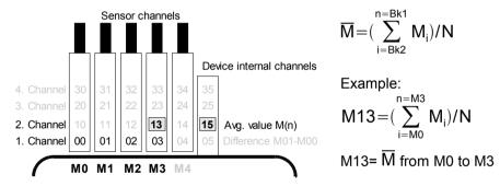
If the sensors are to stay untouched, the function channel can also be programmed to the device internal channels (e.g. M15) (s. 10.3.10). The standard reference channels are here M0 to M1.
