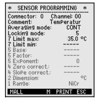
Output of the sensor programming of all active measuring points (command P15 s. man. 6.2.3) with key:
