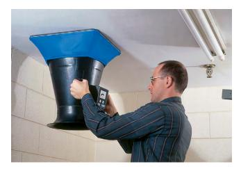
The LoFlo Balometer\* Capture Hood is mainly used in residential or light commercial applications for taking measurements from 10 to 500 cfm (17 to 850 m³/h). The compact size allows them to be used where full size hoods would not fit such as over bathroom stalls or filing cabinets.
